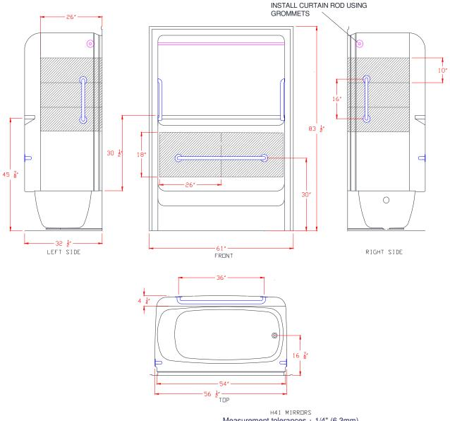
Measurement tolerances  $\pm 1/4"$  (6.3mm)
